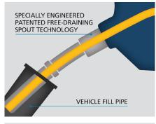
SMOOTH INNER SPOUT BORE. NO DAMS, GROOVES OR RESERVOIRS TO RETAIN FUEL
